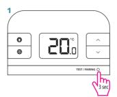
Press and hold TEST / PAIRING button for 3 seconds.
