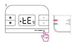
Press TEST / PAIRING button to check the connection with the receiver.
