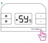
Once devices are successfully paired, LED on the receiver will go solid red. Press and hold TEST / PAIRING button for 3 seconds to end the pairing process.
