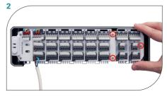
Connect the **CKZM** module to the serial connector.
