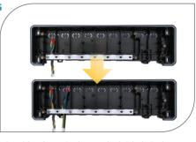
Thread the wires under the mounting belt in the back part of the wiring centre.
