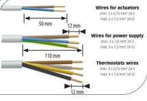
Remove the appropriate pices of insulation from the wires.
