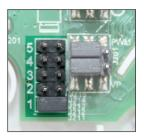
Depending on the amount of actuator used, please change the jumper position accordingly to compensate the power consumption.
