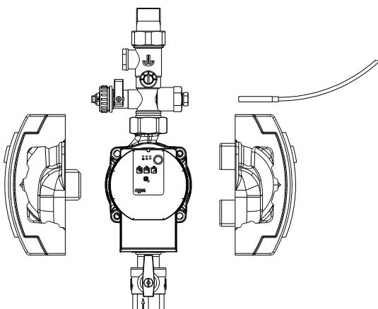
The circulation pump is pre-installed and wired ex works. Connect the power cable of the pump and the temperature sensor cable to the control unit. To do so, refer to the separate operating manual of the control unit and potentially of the supply must correspond to the data given on the type of current and voltage of the mains supply. The type of connection of the pump corresponds to the identification plate.
